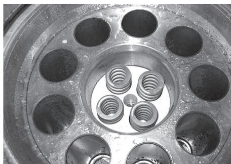
10. Unscrew M8 eye bolt. Place the four springs and spring guide in cylinder barrel. Springs must be positioned in the holes.
