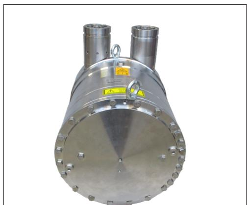
17. Screw in the rest of the bolts and cross tighten all screws to a torque of 30 +/- 2 Nm.
