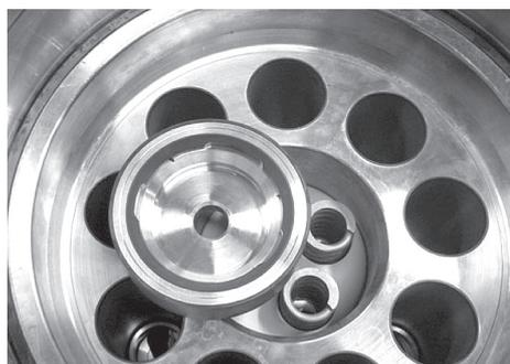
14. Remove the retainer guide, the 4 springs and the spring guide.
