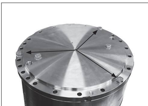
16. Place three bolts in mounting flange. Turn each bolt one round at a time to ensure mounting flange is mounted as straight downwards as possible. Be careful not to squeeze O-ring.
