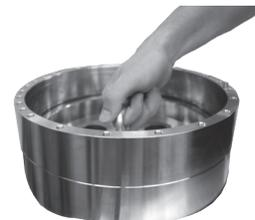
8. Screw eye bolt in cylinder barrel.
