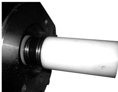
20. Use plastic assembly tool provided with large diameter pointing downwards, to press seal home against shoulder of stop for shaft seal.
