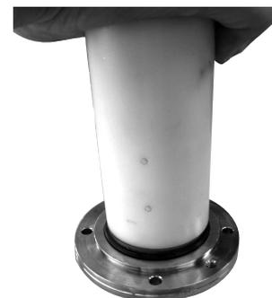
21. Press new ceramic ring into retainer ring by using plastic tool provided.
