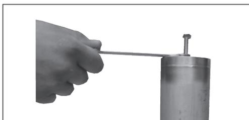
3. Lubricate the new O-rings/back-up rings and the liners in the cylinder barrel with clean filtered water. Lower the valve plate upside down on the cylinder barrel. Place the press bush for valve plate (provided in tool set) like on the picture. Screw the bolt into the shaft of the cylinder barrel. Turn the nut slowly clockwise. The valve plate must slide carefully into the cylinder barrel. Stop when the gap between cylinder barrel and valve plate is 1-2 mm.
