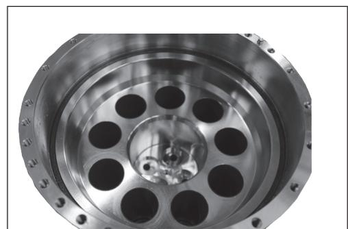
13. Remove the retainer plate and the retainer ball.
