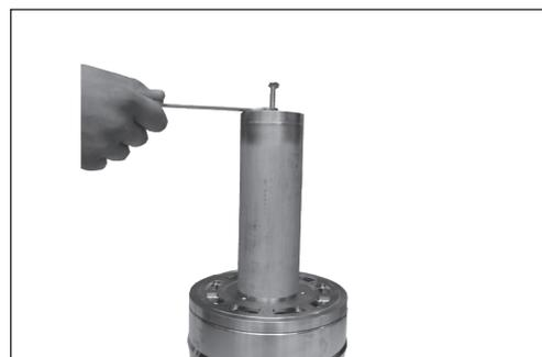
4. Remove the press bush again by screwing the nut counter-clockwise. Turn the nut slowly clockwise. The valve plate must slide gently into the cylinder barrel. Stop when the gap between cylinder barrel and valve plate is 1-2 mm.
