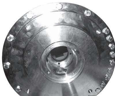
5. Place housing horizontally. Screw in the rest of the screws on port flange. Tighten screws to a torque of  $30 \pm 2$  Nm.
