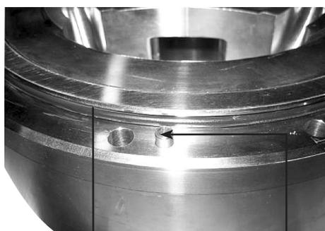
3. Mount O-ring. Insert pin for positioning housing on port flange. Ensure that two screw holes can be reached from below.
