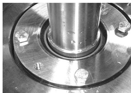
23. Place shaft seal flange on shaft. Tighten the bolts with a torque of 10Nm +/- 2 Nm.
