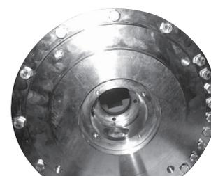
19. Place the pump horizontally. Remove the remaining screws in port flange by using a 13 mm combination wrench. Carefully separate house and port flange. Ensure that pin for the positioning house is not lost.
