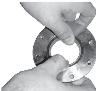
3. Remove ceramic ring from flange by gently pushing it from the back of the sealing ring.
