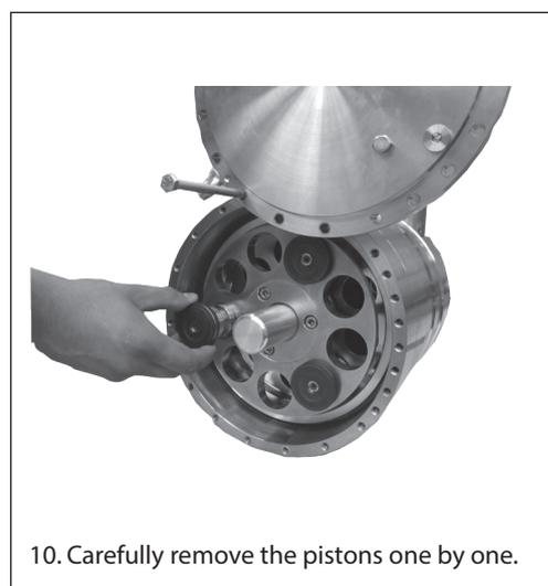
10. Carefully remove the pistons one by one.
