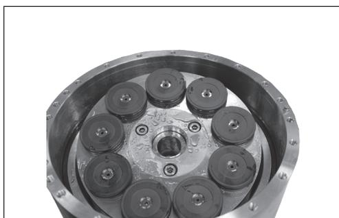
12. Remove by hand the pistons one by one. Be careful not to scratch the pistons. Tilt the retainer plate to horizontal position for easy removal of pistons, if required.
