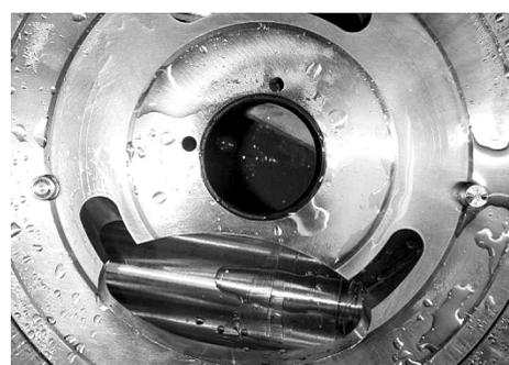
2. Place port flange with O-ring pointing upwards.
