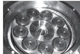
14. Place pistons in retainer plate and cylinder barrel.
