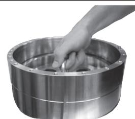
15. Mount a 8 mm eye bolt in the cylinder barrel. Pull straight upwards. A continuous lift will elevate the cylinder barrel out of housing. This can only be done if shaft seal is removed.
