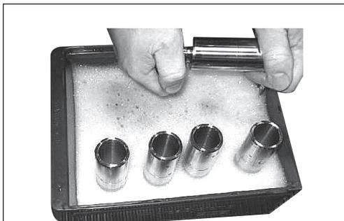
13. Place retainer plate in cylinder barrel.
