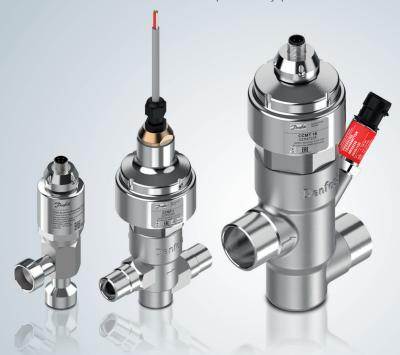
The CCMT is a highly reliable electric pressure regulating valve optimized for transcritical CO<sub>2</sub> refrigeration. The valve has versatile applications in the transcritical system. The valve is capable of high pressure gas cooler control (transcritical). The CCMT can be used as gas by-pass valve (medium pressure control). If desired, the valve can also be used as a normal expansion valve for evaporators.
