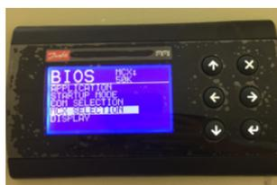
Select "MAN SELECTION" and enter the address of the equipment to which the display is connected (network address).
