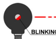
LED RED (blinking) Diagnostic Alarm condition. (relay output contact open) Please proceed replacing the electronic part.
