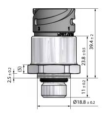
Shown with Bayonet (ISO 15170) connector and M14x1.5 (ISO 6149-2) pressure port.
