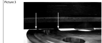
A good way to identify a worn valve plate is to hold a straight knife edge over the valve plate. When holding it up to the light, it will be possible to see any space between the knife edge and the valve plate. See picture 3.
