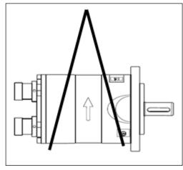
Never use only one sling and make sure the slings does not slip off the pump.
