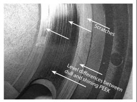
If the port plate has scratches, level differences or both between the arrows, the port plate must be replaced.
