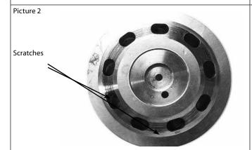
A worn valve plate has scratches, and/or a polished surface. Even small scratches will give a loss of flow.
