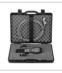
The PFM 100 is used for measuring the differential pressure on both sides of a valve in hydronic systems.
