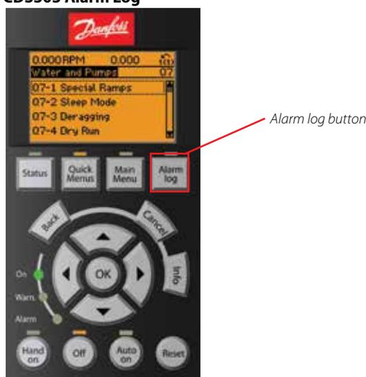
**CDS803 Alarm log (Parameter 15-30 Alarm Log: Error Code)**
