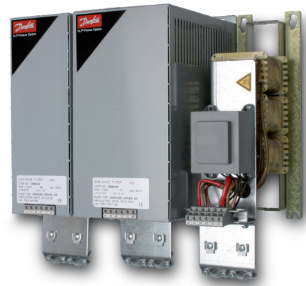
Output filters IP20 (left) or IP00 (right) reduce the peak voltage U_{peak} and the voltage slew rate dU/dt of modern AC drives to protect the insulation of the motor.
