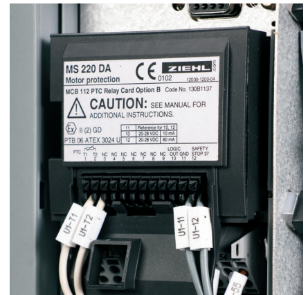
Like all other options of the VLT® AutomationDrive FC 302, the PTC thermistor card MCB 112 can be quickly and cost-effectively retrofitted on site as a plug & play module.
