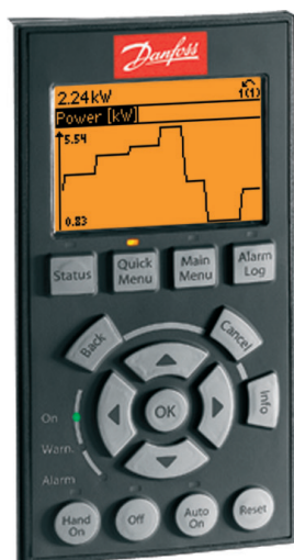
Graphic control panels offer ease of use and information in plain text.
