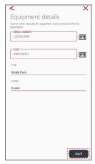
Type or scan the equipment serial number and the code (asset tag/customer code if available). Select the type of the equipment and then the model. The equipment type and model have be communicated in advance to Prosa.
