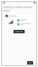
Then the mobile app will show the signal and the network connectivity status. Use this information to verify if the telemetry device is installed properly. Use the Update status button to refresh the information. Registration to the Network should be green as well as the Prosa cloud connection status. For what concern the signal power, it is important to choose the best condition available, considering the instructions reported in the installation user guide.
