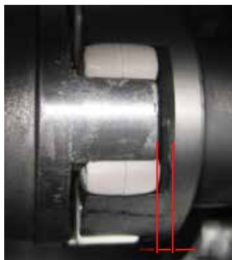
1. Coupling distance (check before disassembling)
