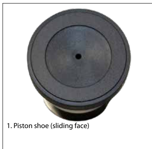
2. Piston shoe (sliding face close-up)
