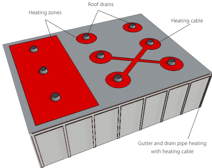
When planning frost protection on flat roofs, protection of the following building elements should be taken into account:
