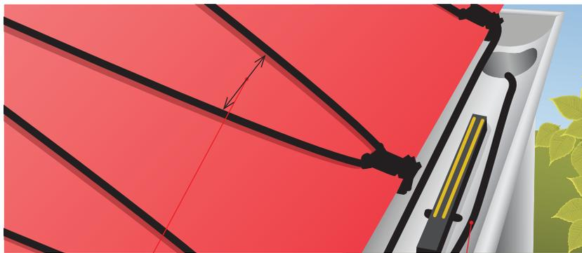
**C-C** – Average cable distance in cm in gutter valleys and on roof areas
