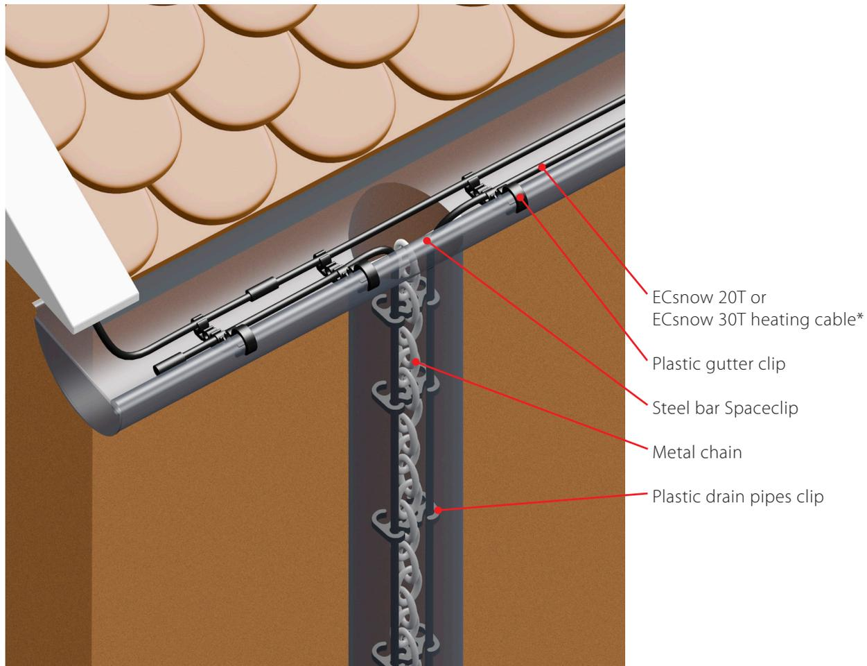
\* For drain pipes with diameter 120 mm or more, two lines of 30 W/m heating cable should be placed. For diameters to 120 mm two lines of 20 W/m heating cable will be enough.
