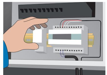
8. Check once again and compare the insulation resistance and Ohm rating for cables. Install ECtemp thermostat and connect cables to the connection boxes and to the switchboard.
