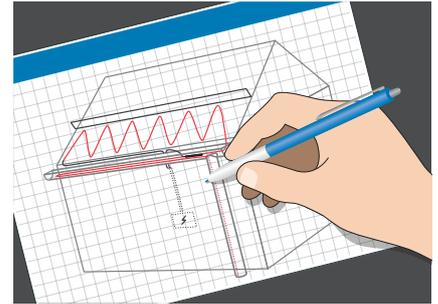
2. Develop the layout plan for cable(s), sensors and thermostats, cable connections/cold tails, connection box, cable paths and a switchboard. Refer to ECtemp 850 manual for location.
