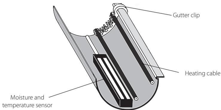
The heating system will be placed in a standard plastic gutter length 37,5 m combined with two drainpipes, with a length of 15 m each. These pipes enter the system sewerage placed approx. 1 m beneath the ground surface.
