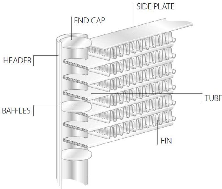
MCHEs have an ingeniously simple design - made entirely of all aluminum which is not only light weight but also prevents galvanic corrosion. The refrigerant-carrying tubes are formed to optimize heat transfer, thus enabling the production of more compact, but equally effective cooling solutions. Meanwhile, their smart louvered fin design maximizes surface contact, successfully reducing the air-side pressure loss, improving efficiency and reducing noise levels.
