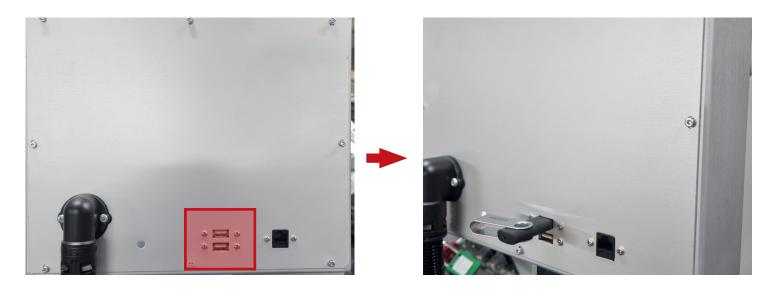
1. Put USB device in the back of the Machine – choose one of the plugs
