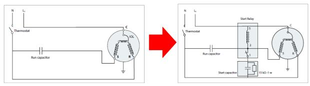
**PSC wiring** with a run capacitor only is the default wiring solution for single phase MLZ compressors.
