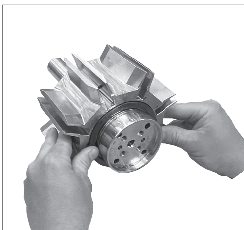
11. Carefully press the rotor element in place.
