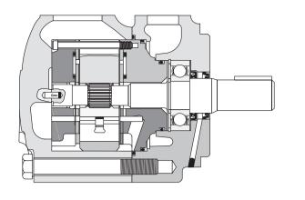
→ TO REVERSE CATRIDGE KIT ROTATION, REMOVE THE TWO (2) 413834 SCREWS, AND REVERSE THE LOCATION OF THE INLET SUPPORT PLATE 430805 AND OUTLET SUPPORT PLATE 419079. REINSTALL THE TWO (2) SCREWS HAND TIGHT. USE PUMP COVER TO ALIGN ALL SECTIONS OF THE CARTRIDGE. REMOVE COVER CAREFULLY AND TIGHTEN SCREWS TO 50 LB. IN. TORQUE.
