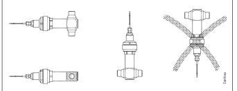
The valve has to be 100% open when mounting - as delivered. The valve must be supported with tube supporters either on the valve itself or on the tubes connected to the valve. The valve must not be exposed to any external influence like shock or punches.
