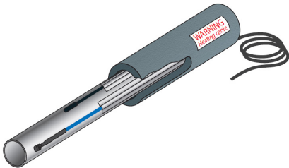
On water pipe installation
