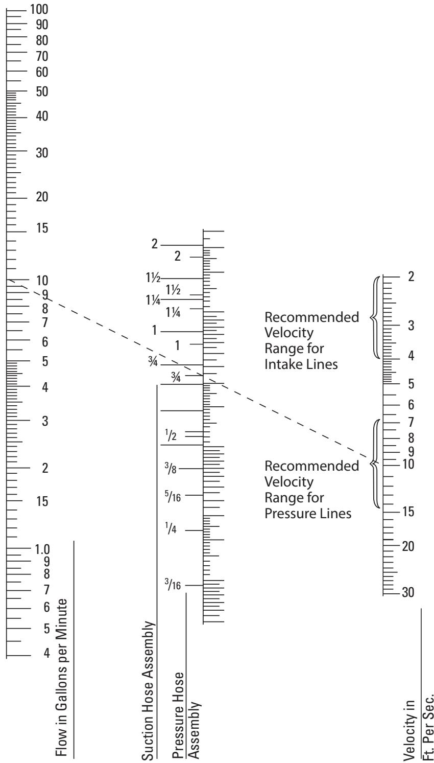
To use Chart 2, lay a straight-edge across the chart as shown by the dotted line. To minimize pressure drop, always use the next larger size hose shown if the line passes between sizes listed.
