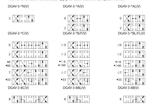
Solenoids identified to U.S. standards (specify "A" in model code) Functional symbols related to solenoid identity "A" and/or "B" according to NFPA/ANSI standards, i.e. energizing solenoid "A" gives flow P to A, solenoid "B" gives flow P to B (as applicable).
