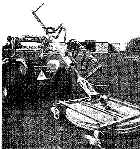
Fig 2. Festooning consists of attaching hose to a steel cable in hanging loops. As one point moves away from the other, the loops open to straighten the hose as needed.
