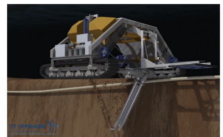
How cables are buried under the sea floor
