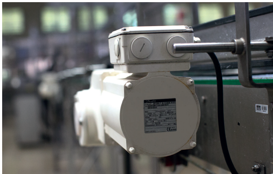
VLT® drives control the speed of the bottling line conveyors, both decentrally ....
