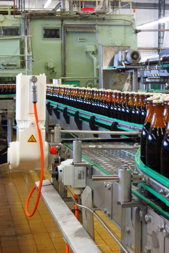
VLT® OneGearDrive® is mounted directly on the conveyor shaft.
