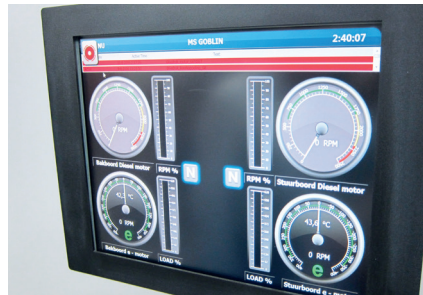
The user-friendly touch screen propulsion control system developed by Hybrid Propulsion System BV.
