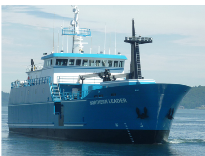
Northern Leader, a state-of-the-art fishing boat, was christened in Seattle, WA, USA, on July 31, 2013. Northern Leader is 184 feet (56 m) long, 42 feet (12.8 m) wide and has a depth of 18.75 feet (5.7 m).
