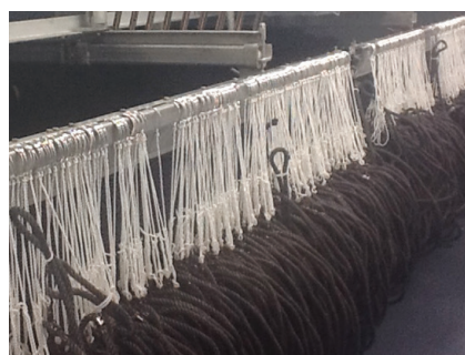
Longline fishing is a commercial fishing technique that uses a long line, called the main line, with baited hooks attached at intervals. The Northern Leader is capable of fishing 76,800 hooks using a Mustad Auto line Super Baiter designed by Mustad Longline AS in Norway. The length of line may stretch to 45 miles (72 km)!
