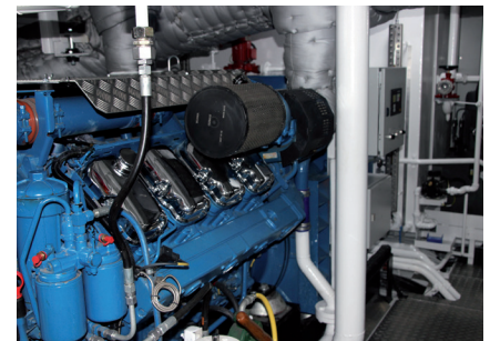
The Scania diesel generators can power the tug during transit and light towing.
