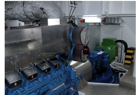
One of the Mitsubishi main engines with the Veth azimuth thruster and the permanent magnet shaft motor/generator. The main engines are used for heavy towing only.
