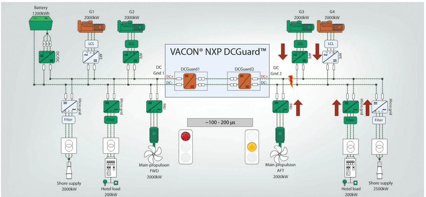
Figure 4 Short circuit situation 0-100  $\mu$ s.
