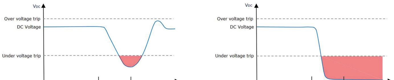
Figure 1 Long fuse clearance time in a DC grid results in a blackout.
