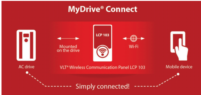
Fig 9.3 VLT® Wireless Communication Panel LCP 103 connecting the AC Drive and Mobile Device
