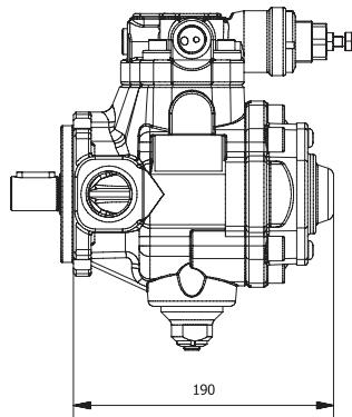
Mounting surface ISO 4401-03 (CETOP 03) for pressure/flow-rate controls CD1/CD2 and CVPD1/CVPD2
