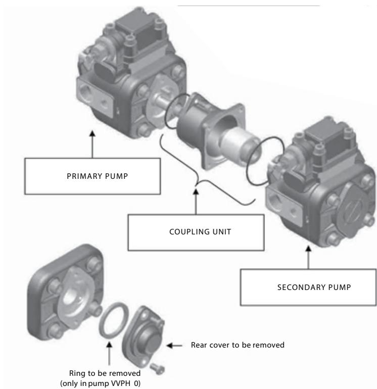
Combined pumps should be mounted in decreasing order of absorbed power, paying attention to the maximum acceptable torque (see diagram on the previous page).
