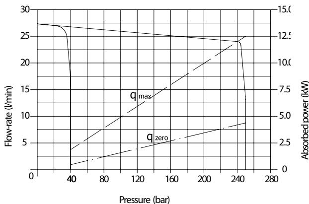
**Drainage (leakage) flow-rate**
