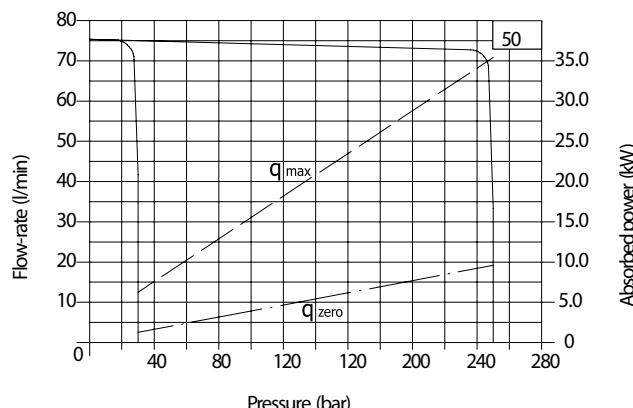
**Volumetric efficiency - zero flow setting curve**
