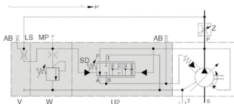
**Load Sensing with Remote Pressure Control "CVPR"****Hydraulic control with load sensing device and remote pressure control**
