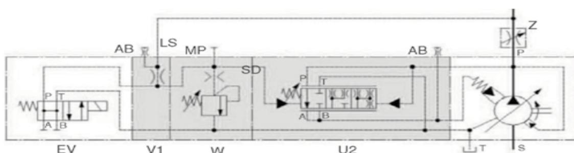
**Load Sensing with Dual Adjustable Pressure Control "CVPD2"****Hydraulic control with load sensing device and two-stage pressure control, one with fixed setting**
