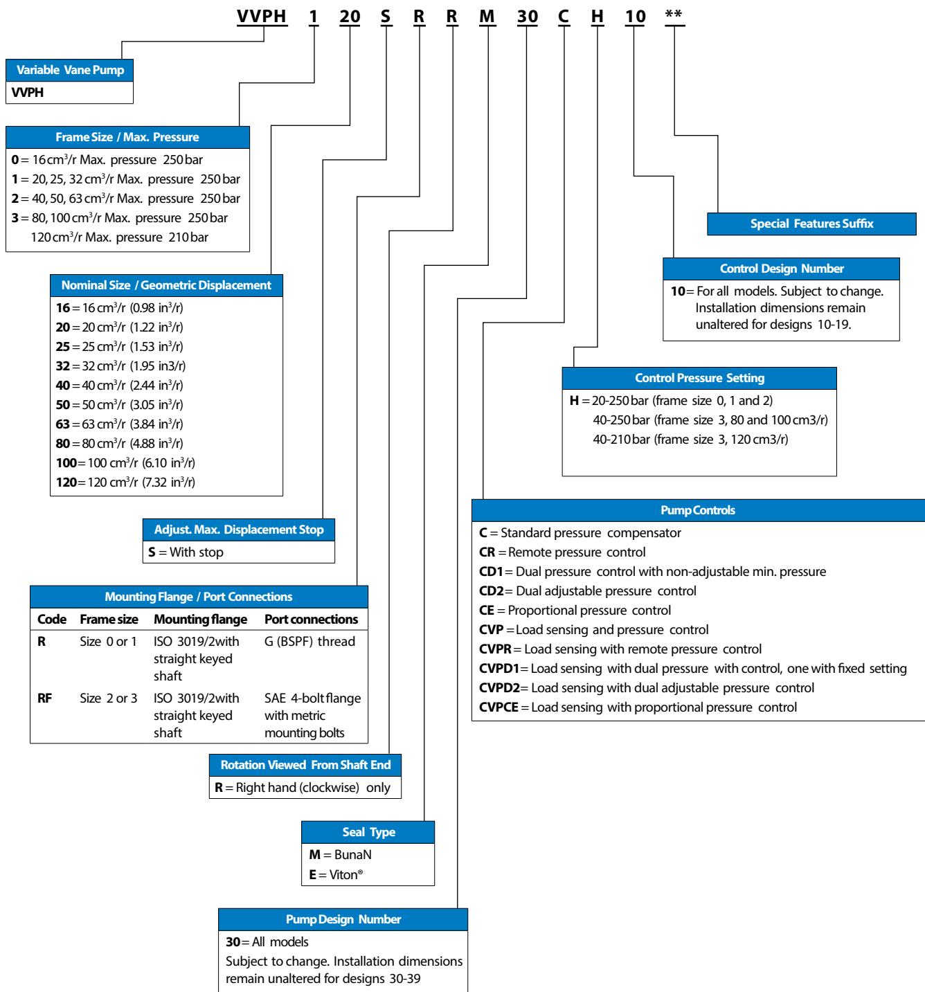
**Note:** See page 33-36 for detailed dimensional listing for mounting flanges, shafts and ports.
