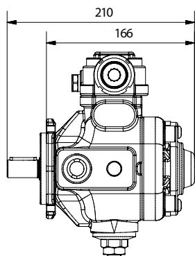
Mounting surface ISO 4401-03 (CETOP 03) for pressure/flow-rate controls CD1/CD2 and CVPD1/CVPD2
