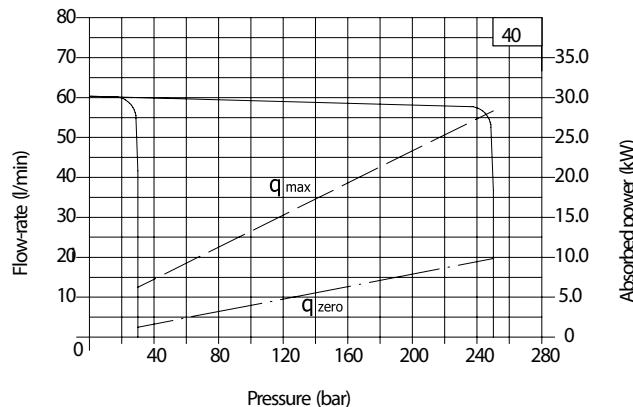
**Volumetric efficiency - zero flow setting curve**
