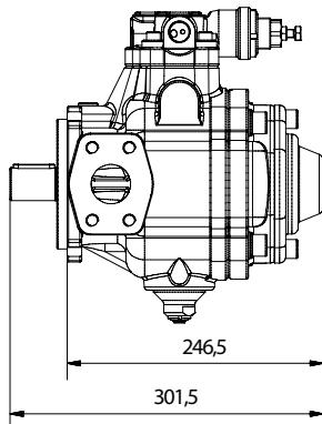
Mounting surface ISO 4401-03 (CETOP 03) for pressure/flow-rate controls CD1/CD2 and CVPD1/CVPD2
