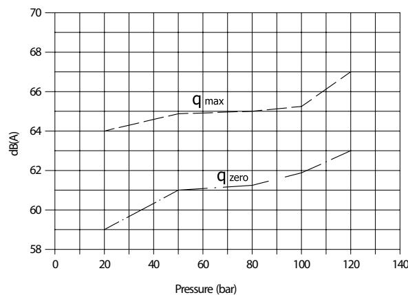
Maximum noise level measured on test rig with sound-level meter placed 1 meter from the pump, with flexible coupling.
