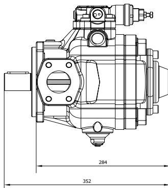
Mounting surface ISO 4401-03 (CETOP 03) for pressure/flow-rate controls CD1/CD2 and CVPD1/CVPD2
