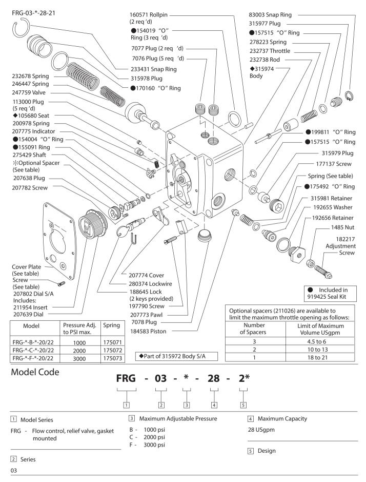
For satisfactory service life of these components, use full flow filtration to provide fluid which meets ISO cleanliness code 18/15 or cleane r. Selections from Danfoss OF P,OFR and OFRS filter series are recommended.
