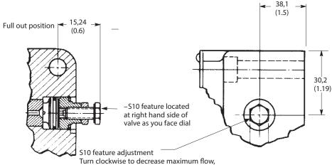
Turn clockwise to decrease maximum flow, Turn counterclockwise to increase maximum flow
