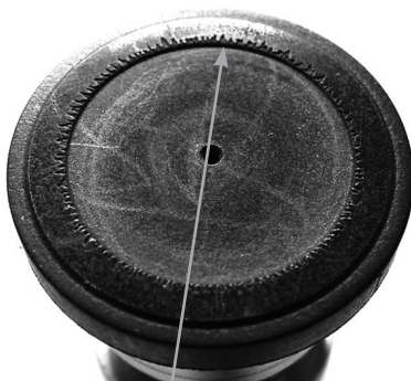
Cavitation of the piston shoes. New inspection is required in 3,000-4,000 hours.
