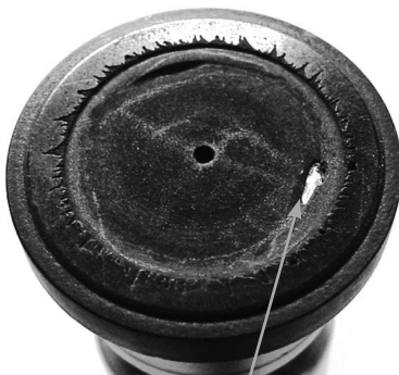
Cavitation of the piston shoes. All pistons must be replaced within the next 100-200 hours.
