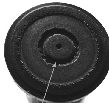
Cavitation of the piston shoes. All pistons must be replaced immediately.
