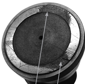
Abrasive wear of the piston shoes. All pistons must be replaced immediately.
