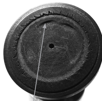
Cavitation of the piston shoes. All pistons must be replaced within the next 500-1,000 hours.
