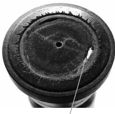
Cavitation of the piston shoes. All pistons must be replaced within the next 100-200 hours.
