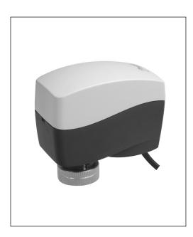
AMI 140 is 2 point 3 wires actuator used with AB-QM (DN 10-32) and VZ, VZL valves. The actuator can be used with fan coil units, induction units, small re-heaters, re-coolers and zone applications in which hot/cold water is the controlled medium. The actuator provides with factory default setting (actuators spindle fully stem down):
