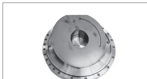
4. Mount the swash plate on the 2 pins. Carefully by hand tilt the unit to horizontal position and mount the 2 bolts which hold the swash plate. Tighten the bolts with a torque according to exploded view. Finally check the surface on the swash plate for any marks or foreign particles.
