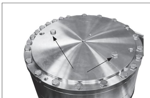
8. Using a 13 mm combination wrench, remove all the bolts on the mounting flange except the three shown in the next picture.
