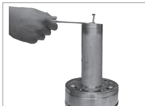
4. Remove the press bush again by screwing the nut counter-clockwise. Turn the nut slowly clockwise. The valve plate must slide gently into the cylinder barrel. Stop when the gap between cylinder barrel and valve plate is 1-2 mm.
