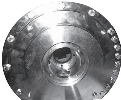
8. Place housing horizontally. Screw in the rest of the screws on port flange. Tighten screws to a torque according to exploded view.
