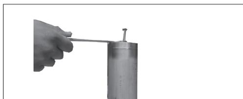
3. Lubricate the new O-rings/back-up rings and the liners in the cylinder barrel with clean filtered water. Lower the valve plate upside down on the cylinder barrel. Place the press bush for valve plate (provided in tool set) like on the picture. Screw the bolt into the shaft of the cylinder barrel. Turn the nut slowly clockwise. The valve plate must slide carefully into the cylinder barrel. Stop when the gap between cylinder barrel and valve plate is 1-2 mm.
