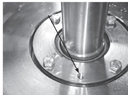
2. Using a 10 mm combination wrench, unscrew the four bolts from shaft seal flange. If shaft seal flange is stuck, screw in two bolts in holes in the flange to remove it.
