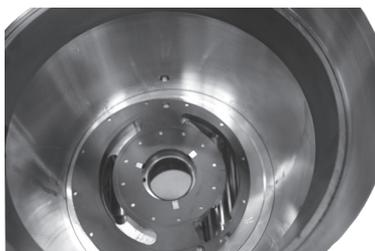
11. Ensure port plate is fitted tightly against the bottom.
