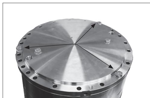
9. Unscrew the remaining three bolts. Turn each bolt one round at the time to make sure that the flange is removed as straight forward as possible.
