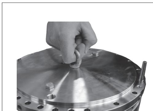
10. Screw the eye bolt in the M8 hole in the middle of the flange. Pull it straight upwards.
