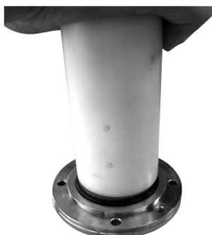
28. Press new ceramic ring into retainer ring by using plastic tool provided.
