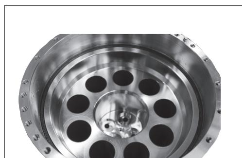
13. Remove the retainer plate and the retainer ball.
