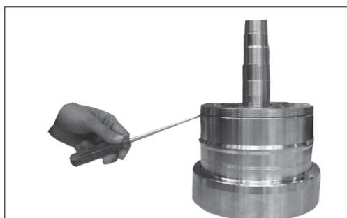
1. Push a screwdriver into the hole between cylinder barrel and valve plate. Carefully push downward the screwdriver so that it makes a gap between cylinder barrel and valve plate. Use this gap to put in another screwdriver and loosen the valve plate from the cylinder barrel.
