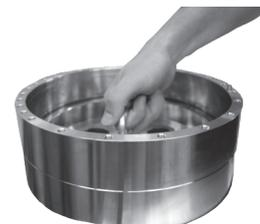
12. Screw eye bolt in cylinder barrel.
