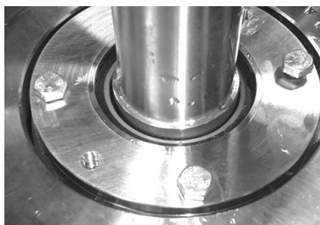
30. Place shaft seal flange on shaft. Tighten the bolts with a torque according to exploded view.
