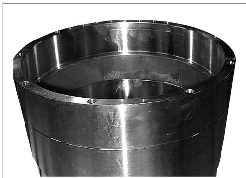
5. Position housing aligning pin hole over guide pin.
