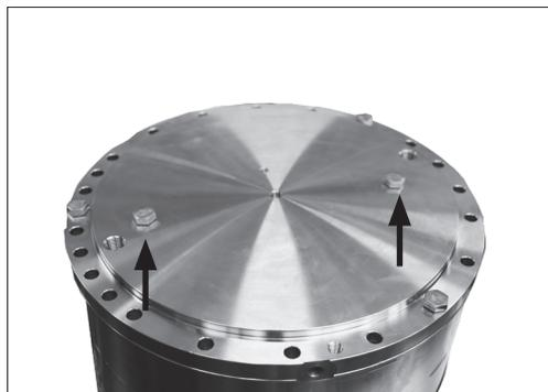
1. Place the swash plate upside down. Remove the 2 bolts holding the swash plate. Remove the mounting flange from the swash plate.
