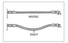
Under pressure, a hose may change in length. Always provide some slack in the hose to allow for this shortening or elongation. (However, excessive slack in hose lines may cause poor appearance.)
