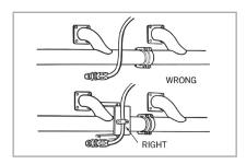
When hose lines pass near an exhaust manifold or other heat source, they should be insulated by a heat resistant boot, firesleeve or a metal baffle. In any application, brackets and clamps keep hose in place and reduce abrasion. For installations where abrasion to the hose cover cannot be prevented with the use of clamps or brackets, a steel protective coil or abrasion resistant sleeve should be placed over the hose.
