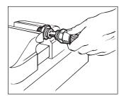
Step 3. Lubricate nipple and socket threads. Use a molydisulfide base lubricant for stainless steel fittings (e.g. MolykoteType G); lubricants containing chloride are not recommended. Other material combinations use standard petroleum lubricants. Hold the nipple with hex in the vise. Push hose over nipple with twisting motion until seated against nipple chamfer. Push socket forward and start threading of socket to nipple.
