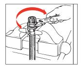
Step 4. Wrench tighten hex until clearance with socket hex is at .031 inches. Your thumbnail is a convenient measuring device. Tighten further to align corners of nip ple and socket hexes. CLEAN, PROOFTESTTOTWICE OPERATING PRESSURE AND INSPECT ALL ASSEMBLIES.
