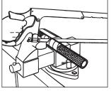
**Step 1.** Cut hose square to length with fine-tooth hack saw or cut-off wheel. To minimize wire braid flare out, wrap hose with masking tape and cut through tape. Remove tape, trim loose wires and flush with lube before next step. Burrs on bore of tube should be removed with a knife. Clean the hose bore.
