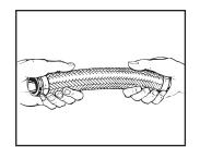
**Step 2.** Stretch until snug, mark length and cut with tin snips.
