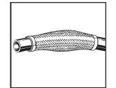
**Step 1.** Disconnect the ra diator hose. Slide overbraid over the radiator hose.
