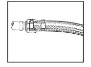
**Step 2.** Push cap (socket) onto hose until it bottoms. Then slide clamp under cap.
