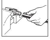
Step 2. Push hose on fitting until hose end bottoms under neath protective cap as shown. Clean, proof test to twice oper ating pressure and inspect all assemblies.
