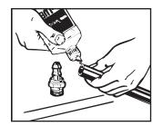
Step 1. Cut hose to required length with a sharp knife. Oil inside of hose and out side of nipple liberally.
