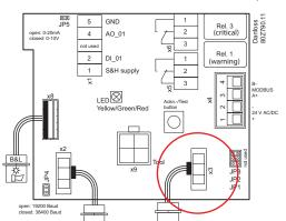
Sensor head connection. The sensor can be replaced in case of failure or end of life of the sensor.
