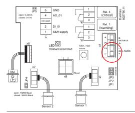
If Modbus communication is used, X4 3 and 4 have be wired.
