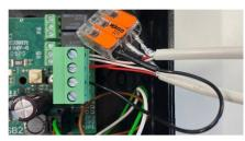
If the Analog Output is used, X1 4 and 5 have to be wired. The same ground potential for the AO and the connected device is required.
