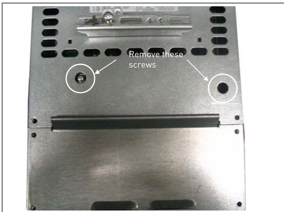
Figure 5-8. Changing of EMC protection class, MF6
