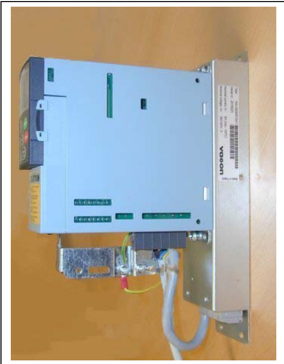
Figure 6-10. MF2 with the RFI-filter RFI-0008-5-1
