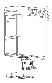
**Step 4**Fit bottom cover onto frequency converter and tighten an M4 X 10 screw.
