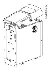
**Step 2**Install clamps onto metal bracket and tighten M4 X 20 screws.
