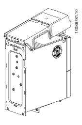
**Step 2**Mount metal bracket onto frequency converter and tighten two M4 X 10 screws.
