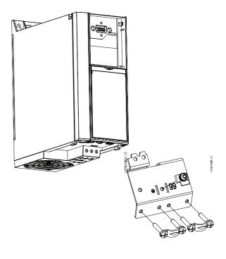
**Step 2**VLT Micro Drive FC 51 mounted with de-coupling plate
