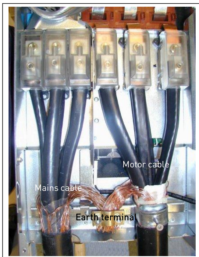
Figure 6-17. Cable installation in Vacon NXS/P, FR8
