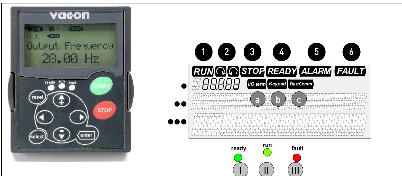
Figure 7-1. Vacon control keypad and drive status indications
