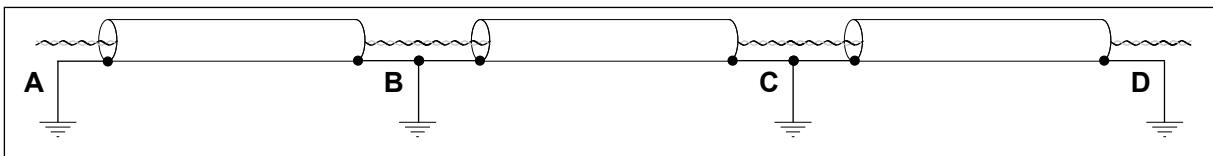
Fig. 38: Grounding in noisy environment with good equipotential. If potentials at points A, B, C and D are very different and cannot be made similar, cut the shields as in Fig. 39.
