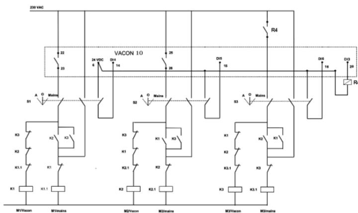
Figure 6.2: 3-pump autochange system, sample control diagram
