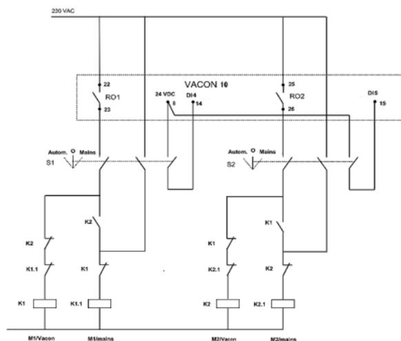
Figure 6.1: 2-pump autochange systems, sample control diagram
