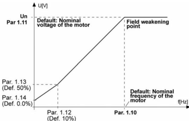
Figure 10.2: Programmable U/f curve
