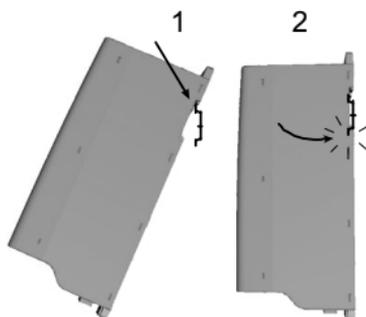
Figure 3.2: DIN-rail mounting, MI1 - MI3
