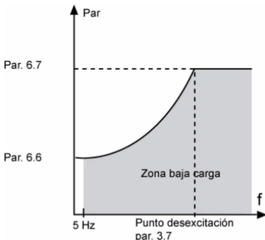
Figure 10.4: Setting Minimum Load
