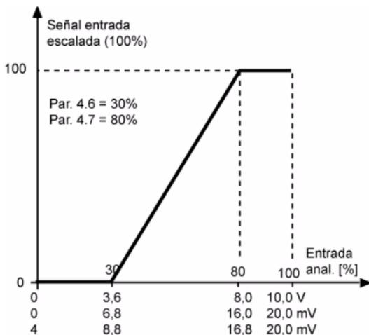
Figure 10.3: Example of signal scaling
