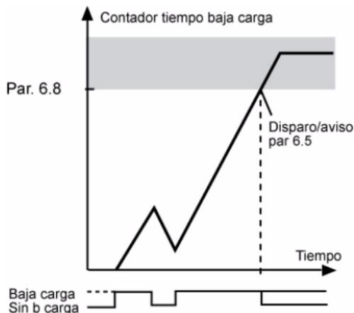
Figure 10.5: Underload Timer Function
