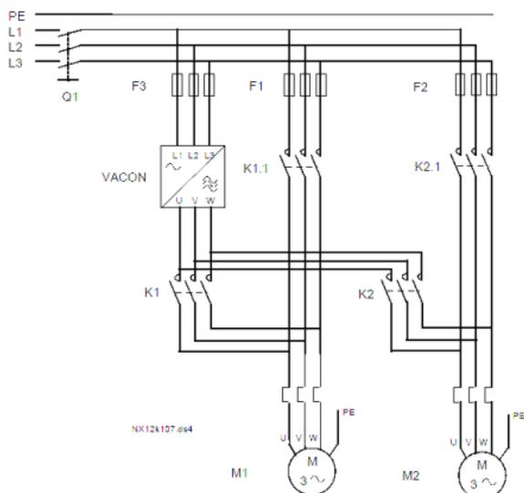
Figure 6.3: Example of 2-pump autochange, power diagram
