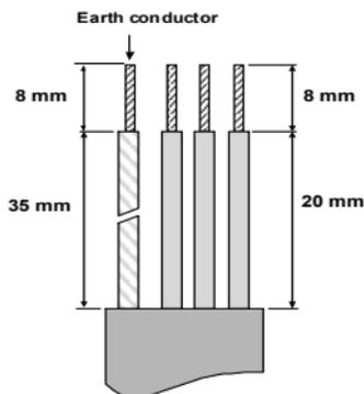
Figure 3.15: Stripping of cables
