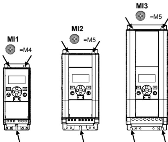
Figure 3.1: Screw mounting, MI1 - MI3
