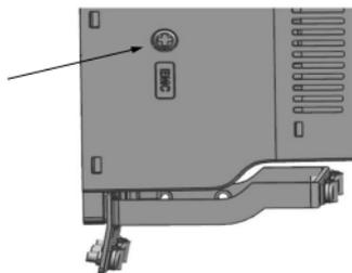
Figure 3.6: EMC protection class, MI1 - MI3
