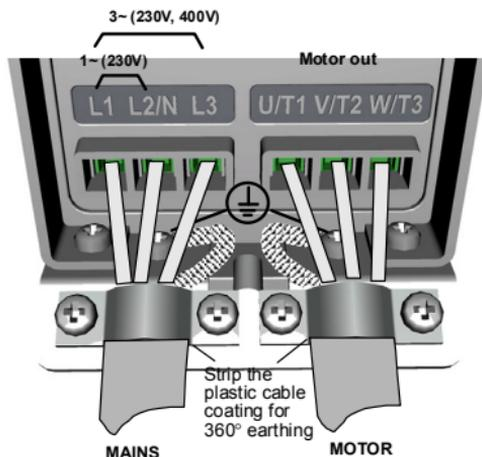
Figure 3.7: Vacon 10 power connections, MI1
