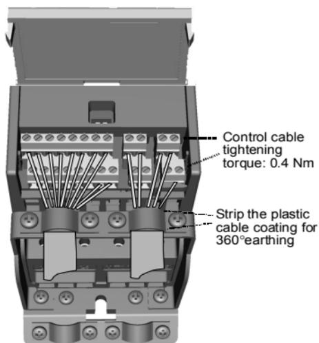
Figure 3.11: Install the control cables. MI1 - MI3. See Chapter 6.1
