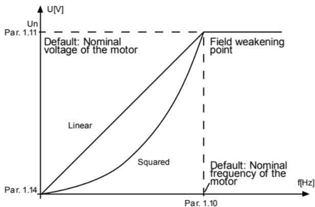
Figure 10.1: Linear and motor voltage change
