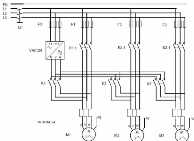
Figure 6.4: Example of 3-pump autochange, power diagram
