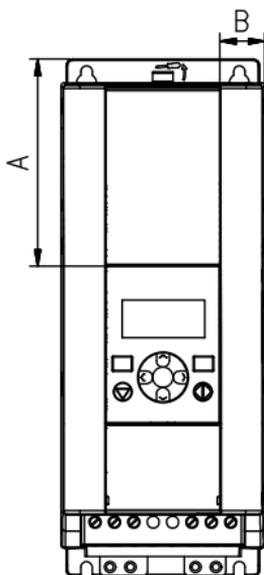
Figure 3.4: Vacon10 dimensions, MI2 - 3 Display Location
