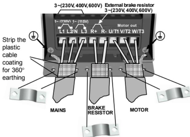
Figure 3.8: Vacon 10 power connections, MI2 - MI3
