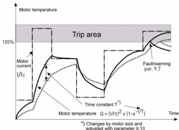
Figure 10.7: Motor temperature calculation
