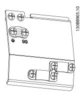
**Step 3**VLT HVAC Basic Drive mounted decoupling kit.
