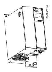
**Step 2**Mount decoupling kit on frequency converter and fasten it with 2 screws. Tightening torque: 2Nm.
